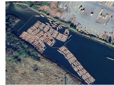
Figure 81 Aerial imagery of a log storage area, with horizontal logs line the edges of this inlet as a 'log barrier'. Neither of these features should be digitized as log accumulation. Imagery ©2025 Airbus via Google Earth Imagery 10/10/2022.
