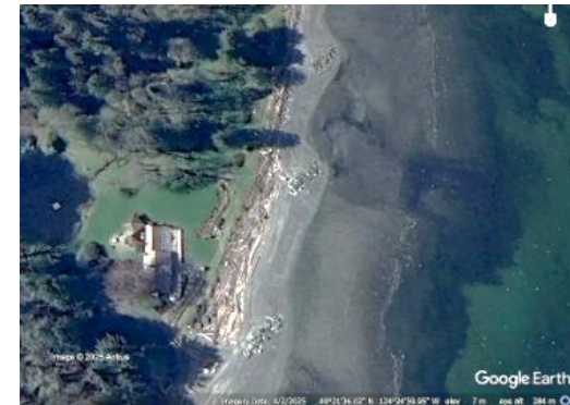
Figure 6 An example of an exception to the rule - groynes built in the intertidal, with a substantial portion of the construction existing in the high intertidal zone. Image © 2025 Airbus via Google Earth imagery date: 4/2/2025.
